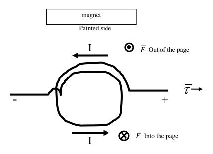
From this diagram you should be able to determine that the top of the coil is coming out of the page, and the bottom of the coil is going into the page. Applying  $\overline{F} = I\overline{L} \times \overline{B}$  at the very top and very bottom of the coil, it can be determined that the magnetic field,  $\overline{B}$ , supplied by the magnet is pointing down; therefore, the painted side of the magnet is the North Pole of the magnet.
